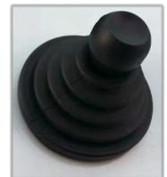
**CAUTION:** Before handling any pilot, pulling, or conductor lines attached to this machine, the operator must ensure that the hydraulic drum brake is set by releasing the joystick.
