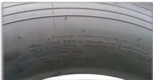
**CAUTION:** Replacement tires must meet the same specifications as the originals. Tires for Sherman+Reilly™ machines meet specific duty requirements, as well as weight and roadway/speed ratings. Mismatched tires and rims may come apart with explosive force causing personal injury. Mismatched and underrated tires can also blow out causing vehicle and roadway accidents that can create serious injury or death for those involved.
