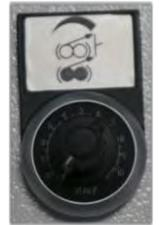
**NOTE:** If operations must be stopped and the line/bullwheels, for whatever reason, do not stop when the puller on the other end stops pulling; the operator can increase the tension until the bullwheels slow to a stop and hold the line. Once the bullwheels are stopped, press the Pull Mode button. If using Sync Tension Mode (A, C, or D), push the Sync Tension Mode Off Button to stop and set the brake. Ensure the tension setting is readjusted prior recommencing tensioning operations.
