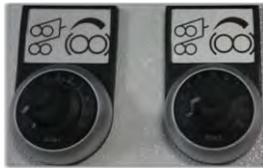
**NOTE:** The Master Sync Mode Bullwheel Potentiometer can be used to control all bullwheels at once. These potentiometers allow additional individual tension adjustments.
