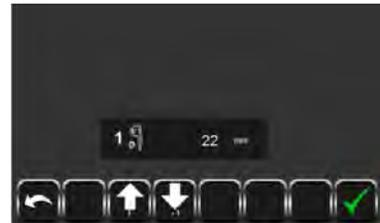
Once the diameter is showing the correct value, press the green checkmark button to save the new setting and return to the Client/Service menu.
