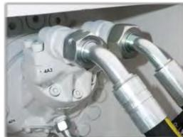
**WARNING** Never check for hydraulic leaks with hands or body. When under pressure, leaks can penetrate the skin. Small or pinhole size leaks may be invisible during visual inspection. (Using a piece of cardboard or wood is recommended).
