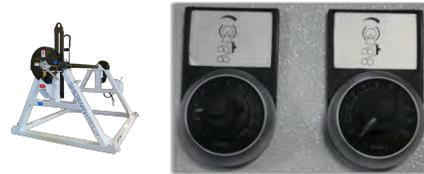
**CAUTION:** Rotate reel potentiometers slowly, and ensure all personnel are clear of the area and aware of rope take-up. Rapid increases in reel tension can create large jolts in the line and possible equipment or conductor damage.
