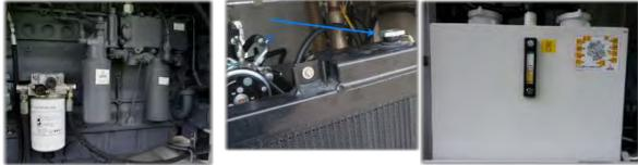
**NOTE:** It is necessary to open the engine covers to check the fluid levels. Be sure all covers are closed and latched in position properly before transport or operating the machine.
