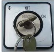
**NOTE:** After the key switch is turned to the [ON] position, the system will begin a start-up phase, where the computer system boots up, and the ventilators, button lamps, and circuits are tested. This process takes approximately 30 seconds.
