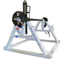
**WARNING:** If the reel control potentiometers have a positive setting at the time the machine starts, any connected reels will automatically begin to rotate to apply the preset tension. This can create unanticipated line jolts as well as life threatening or severe bodily impacts to surrounding personnel if they are not aware of the line/conductor take up and/or reel spin.
