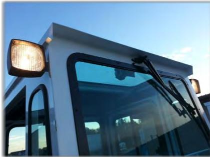
**NOTE:** The master power key switch must be turned to the on position to activate the exterior work lights.
