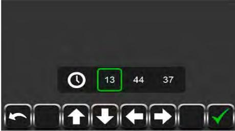
To change the time in the system, use the right and left arrow buttons to move the green selection box between Hour, Minute, and Second intervals. Once an interval is selected, use the Up and Down arrow keys to adjust the number up or down.
