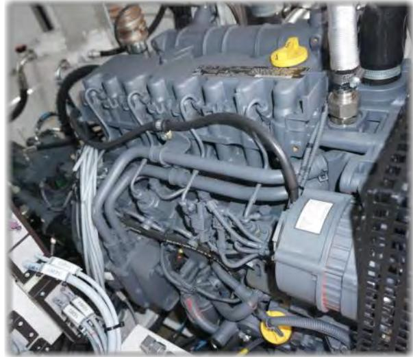
**CAUTION:** Never add ETHER to fuel to start cold engine. Ether WILL damage diesel engines. Use available heater system as needed.
