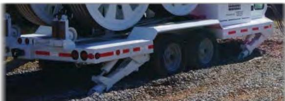
**CAUTION:** All jacks must be extended for stabilization, and the machine must be leveled prior to conduction operations.
