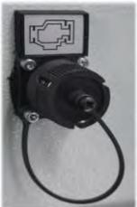
**NOTE:** The data port has two metal pins on the top to allow the data cable to be locked in place. This helps prevent the cable from unintentionally becoming detached during diagnostics.
