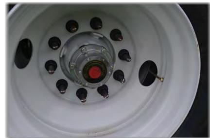
**CAUTION:** Wheel nuts or bolts must be tightened and maintained at the proper torque levels to prevent loose wheels, broken studs, and potential dangerous separation of the wheel from the axle, which can cause accidents, personal injuries, and death.
