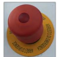
**NOTE:** The emergency stop button should only be used to stop the machine in an emergency situation where there poses a risk of injury or death to personnel or to prevent equipment or property damage. When this button is pushed, line tensions can change rapidly. For more information on emergency shutdown situations- (see the Emergency Stop Procedure).
