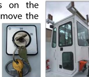
**NOTE:** It is important that the windows are closed, the door is locked, and that all keys are removed to prevent unauthorized access or tampering with the equipment, especially when the machine is parked in a publically accessible area or area adjacent to a roadway or construction site.
