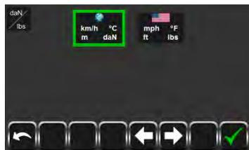
The two options are metric/decimal-(Globe) and non-metric/customary-(USA Flag). This setting change is a global change for the system, meaning that it will affect all system displays where units of measure are displayed. Additionally, this setting will also change how the data is recorded. Once the data is recorded for an operation under one UOM, it cannot be changed in the system.
