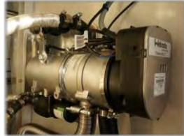
**NOTE:** The arctic kit is an optional equipment add-on to assist with warming the machine engine components when operating in very cold temperatures. **This option may not be installed on all models. If not installed, skip this step.**
