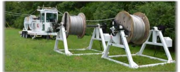
**NOTE:** The reel stand hydraulic controls should be in the disengaged or Off/Closed position when not in use.
