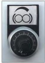
This potentiometer is used to regulate the amount of tension applied by the bullwheels. When setting the amount of tensioning force, rotate the knob CW to increase and CCW to decrease.
