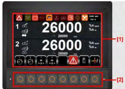
on and the system loads, the first screen the operator sees (after the S+R™ logo screen) is the **MAIN MENU screen**. This screen allows the operator to access the functions of the system, while also allowing access to settings and diagnostics.
