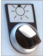
This switch when turned CW will turn on the exterior work lights.
