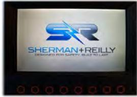
The system control panel has eight backlit soft key buttons for control of machine and computer functions. The panel is also
