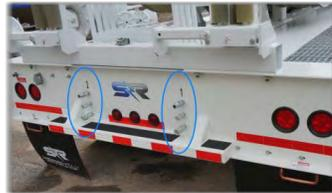
**NOTE:** Always ensure that the hydraulic hoses are properly secured to the quick release ports at both ends prior to starting the engine, and prior to engaging hydraulic circuit. Residual pressures existing in the hydraulic lines, even with valve Off, can inhibit connecting hose.
