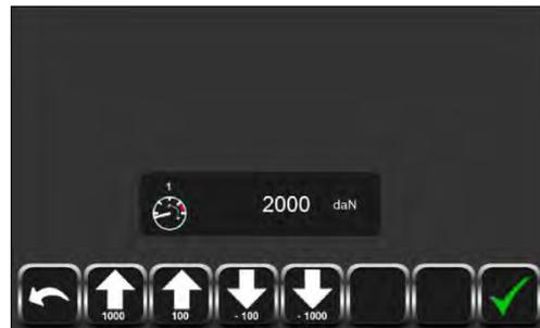
To increase or decrease the amount, press the UP and DOWN arrow buttons. The operator can increase or decrease the amount in increments of 100 or 1,000.
