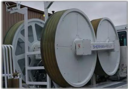
**CAUTION:** Before pushing the ATS/Tension Mode Selection Button a second time, the operator must set the pre-tension for the line. Otherwise, as soon as the ATS/Tension Mode is engaged (button pushed a second time), the bullwheels will begin to apply tension at the current potentiometer setting. This can create either a sudden rise or drop in tension.
