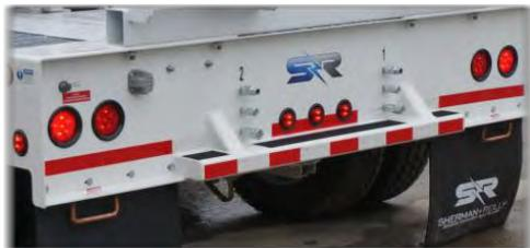
**CAUTION:** Do not tow the machine/unit unless all the trailer lights and brakes are working correctly.
