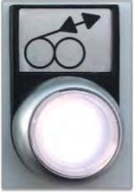
This control button, when pushed, engages the line pulling mode for the machine. When this button is pressed, the button backlight will illuminate, indicating that the system computer has changed over to Pull Mode.
