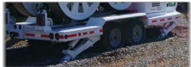
**CAUTION:** Ensure that all jacks are fully raised and clear of the ground before attempting to tow trailer.
