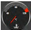
The gauge on the far right displays the engine coolant temperature.
