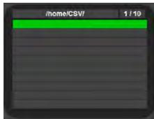
This section displays the recorded data stored in the system computer memory. Stored data will show with the file name of the record consisting of the machine number with the bullwheel number, the current date, and a two-digit counter number. A new file is created each time recording is initiated.
