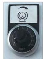
**CAUTION:** Rotate reel potentiometers slowly, and ensure all personnel are clear of the area and aware of rope take-up. Rapid increases in reel tension can create large jolts in the line and possible equipment or conductor damage.
