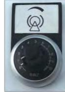
This potentiometer is used to regulate the amount of tension/braking pressure applied by the hydraulic reel stand.
