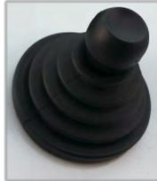
**NOTE:** If the joystick is released, it will return to the center neutral position, the bullwheel rotation will stop, and the hydraulic brake will set.
