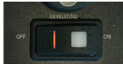
4. Turn off the automatic levelwind control using rocker switch in the cab.
