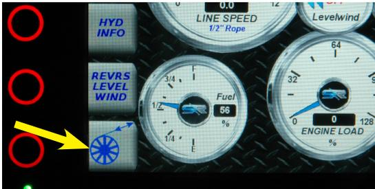
The **POWER mode** is also used when assisting with unspooling line from the drum, and will use hydraulic pressure to “drive” the line at a determined speed and resistance. This is controlled with the joystick.
