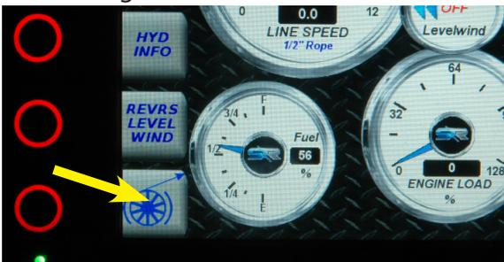
The amount of **LINE DRAG** that is applied is controlled with the joystick.
