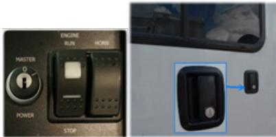
**NOTE:** It is important that the windows are closed, the door is locked, and that all keys are removed to prevent unauthorized access or tampering with the equipment, especially when the machine is parked in a publicly accessible area or area adjacent to a roadway or construction site.
