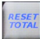
When this button is pushed and held for three seconds, it will reset the footage counter to zero. The footage counter is displayed at the top center on the HOME screen.
