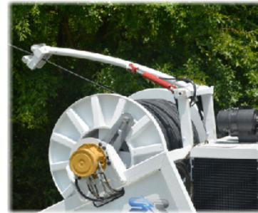
**CAUTION:** Line of sight view of the jacks and levelwind should always be established prior to operating these components using the outside hydraulic control panel. Operators should first ensure that all personnel are clear of the area.
