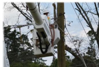
To provide slack, depress the joystick trigger then pull back slightly on the joystick, bringing it out of neutral. Then pause for about three seconds for the brake to release. Once the brake releases, with the joystick trigger still depressed, cross over neutral by pushing the joystick forward.
