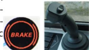
**WARNING:** To avoid potential personal injury and/or equipment damage, ensure that any vehicle actively pulling out line has completely stopped before returning the joystick to the center neutral position and setting the brake. Limit pull off vehicle speed to account for sudden accidental changes in line tension.
