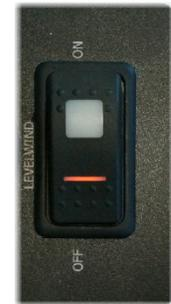
6. Ensure that the levelwind float arm is set to ON.
