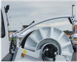
The levelwind can be manually operated, if needed, using the joystick, outside panel, and manual override controls; however, the levelwind is designed to operate
