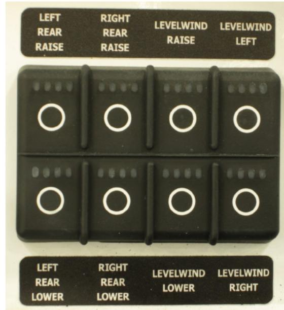
To operate the control, simply push and hold the button to move the machine component. When the button is released, the motion will stop. All buttons are labeled with their corresponding function and motion direction.
