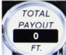
**NOTE:** The footage counter should only be reset when the line is all the way out from or onto the drum. Otherwise, the values will not accurately represent how much line is on/off the drum.
