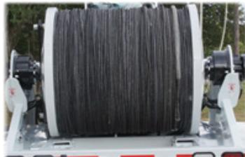
Then, using a tie-off rope around the drum, secure the rope end to the drum.
