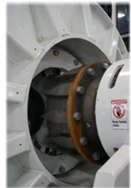
**NOTE:** If sides are not fully retracted and the drum coupler is not fully seated, the system will not allow drum rotation. The system monitors the drum engagement to ensure that both sides are safely seated prior to allowing drum rotation operations.
