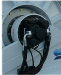
By default, the drum brake will be ON when the machine is started up. To disengage the hydraulic drum brake, depress the joystick trigger then pull the joystick slightly backward and out of neutral. It may take a few seconds for the system to build up hydraulic pressure before the brake is released and the drum will begin to spin. Returning the joystick to center without the trigger depressed will activate the brake.
