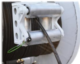
4. If not completed already, have the cable end and the conductor pulling grips attached to opposite sides of swivel on the conductor side.
