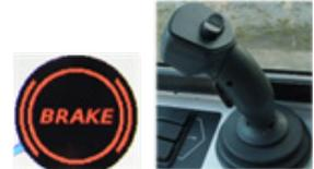
**CAUTION:** Before handling any pilot, pulling, or conductor lines attached to this machine, the operator must ensure that the hydraulic drum brake is set and the joystick is in the neutral position with the joystick trigger released.
