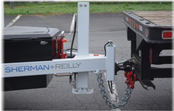
9. Slowly retract trailer nose/hitch jack, so that the pintle eye goes over and rests correctly on hitch.
