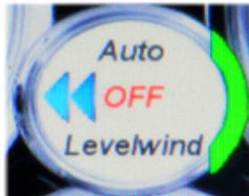
**NOTE:** The operator will need to set the initial direction (Right/Left) of the levelwind before beginning operations. The direction will depend on which side of the drum the rope end leading off is located.
