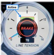
**NOTE:** The tension limits can be changed without halting operations by using the rotating control knob on the display.
