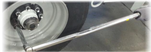
**CAUTION:** Wheel nuts or bolts must be tightened and maintained at the proper torque levels to prevent loose wheels, broken studs, and potential dangerous separation of the wheel from the axle, which can cause accidents, personal injuries, and death.
