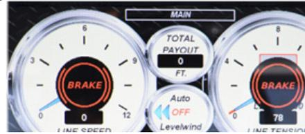
**NOTE:** To stop drum rotation at any time, return the joystick control to the center neutral position **with the joystick trigger released**, and the hydraulic drum brake will set.
