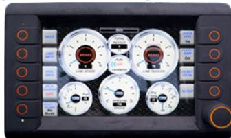
**NOTE:** Warnings and faults are displayed as a red icon or button. If warnings or faults are present, see the faults and diagnostics screens, and check system components prior to beginning operations- (see *General Faults in the TROUBLESHOOTING* section).
