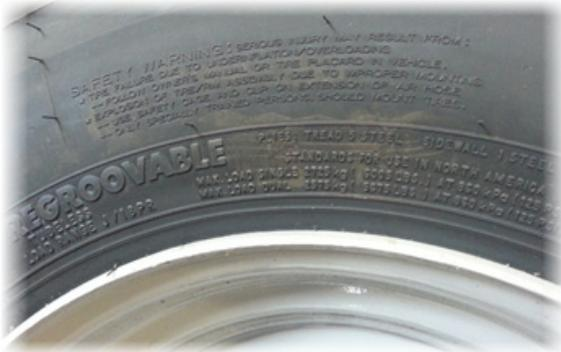
**CAUTION:** Replacement tires must meet the same specifications as the originals. Tires for Sherman+Reilly machines meet specific duty requirements, as well as weight and roadway/speed ratings. Mismatched tires and rims may come apart with explosive force causing personal injury. Mismatched and underrated tires can also blow out causing vehicle and roadway accidents that can create serious injury or death for those involved.
