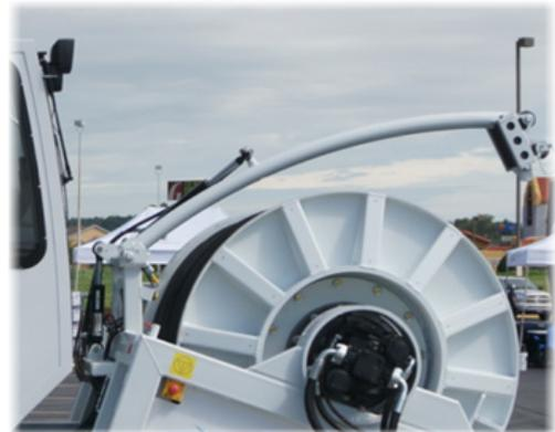
8. The system will now automatically manage the levelwind functions. The operators can adjust the speed of the levelwind, if needed, by rotating the levelwind speed control knob clockwise (CW) to increase speed and counter-clockwise (CCW) to decrease speed.
