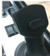
2. Using the top joystick lateral rocker switch, adjust the R/L starting position of the levelwind so that the levelwind is centered over the exit rope.
