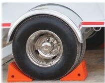
6. Chock wheels on both sides of the machine/unit trailer, then start machine/unit engine- *(See Start-Up Procedure section)*.
