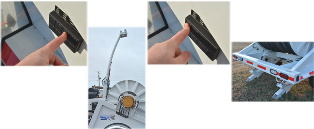
**CAUTION:** Line of sight view of the jacks and levelwind should always be established prior to operating these components using the outside hydraulic control panel. Operators should first ensure that all personnel are clear of the area.
