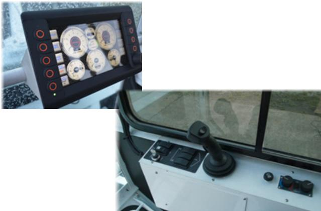
A 12-Volt DC power port has been provided on the operator control console. This port can be used to charge field radios or cellular telephones, or provide power for other similar devices.
