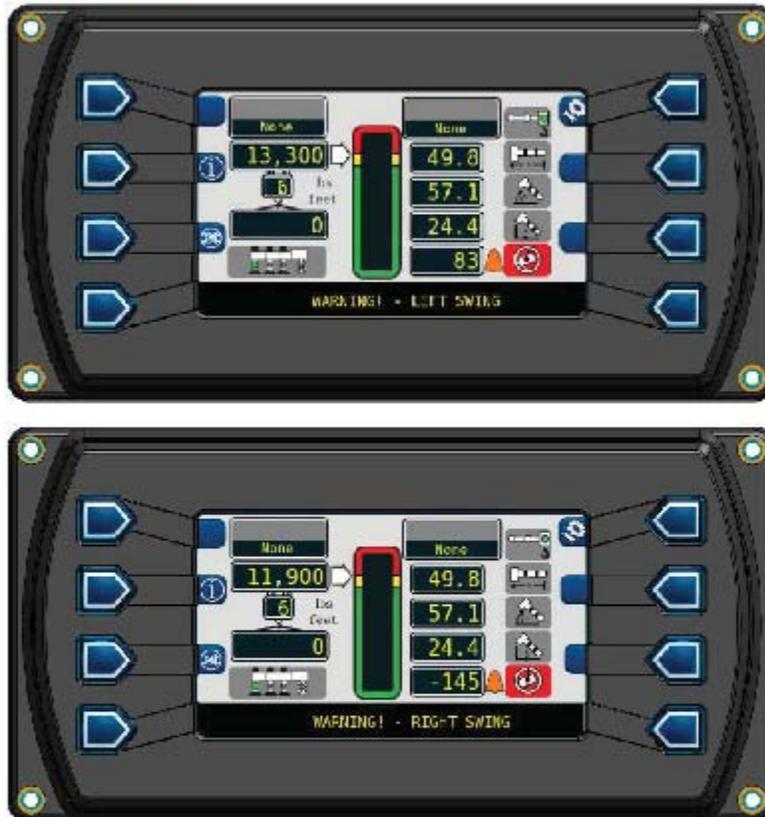
*Note: The user set swing alarm will not result in a function kick-out, (FKO) when triggered.*
