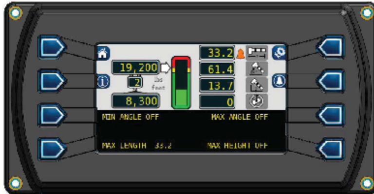
4. Pressing the MAX LENGTH button again, will cancel the alarm, and the display will read: MIN ANGLE OFF.
