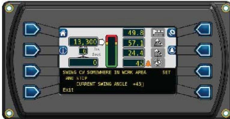
6. Rotate the boom to the right swing point and press the key adjacent to "OFF."
