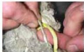
To determine the extent of outer fiber damage from abrasion, a single yarn in all abraded areas should be examined. The diameter of the abraded yarn should then be compared to a portion of the same yarn or an adjacent yarn of the same type that has been protected by the strand crossover area and is free from abrasion damage. (LEFT)
