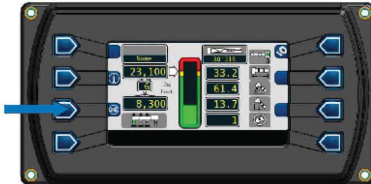
The audible alarm remains cancelled until the condition which caused the alarm has been resolved.
