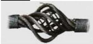
A "birdcage" is caused by sudden release of tension and the resulting rebound of rope. These strands and wires will not be returned to their original positions. The rope should be replaced immediately.
