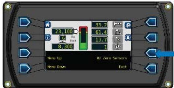
*Note: The boom must be completely collapsed in order for the zero point to be accurate on the display.*
