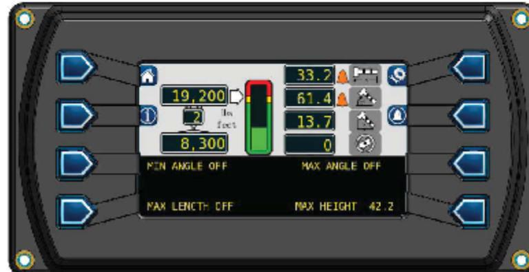
4. Pressing the MAX HEIGHT button again, will cancel the alarm, and the display will read: MAX HEIGHT OFF.
