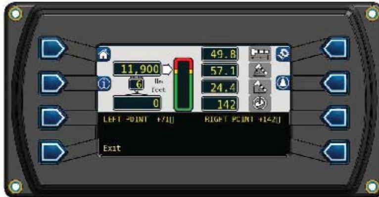
5. Rotate the boom to the right by raising or retracting the boom, or raising the load above the obstacle until the right point is reached. Or, rotate the boom to the left until the right point is reached (this will avoid having to pass through the exclusion zone). This will be the point to the right facing the exclusion zone to be defined.
