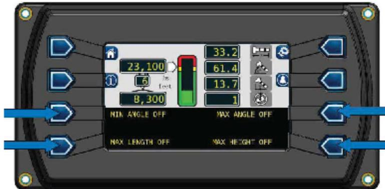
There are four buttons to the left and right of the home display screen. Each button relates to the alarm to which it is pointing.
