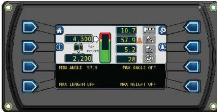
4. Pressing the MIN ANGLE button again, will cancel the alarm, and the display will read: MIN ANGLE OFF.
