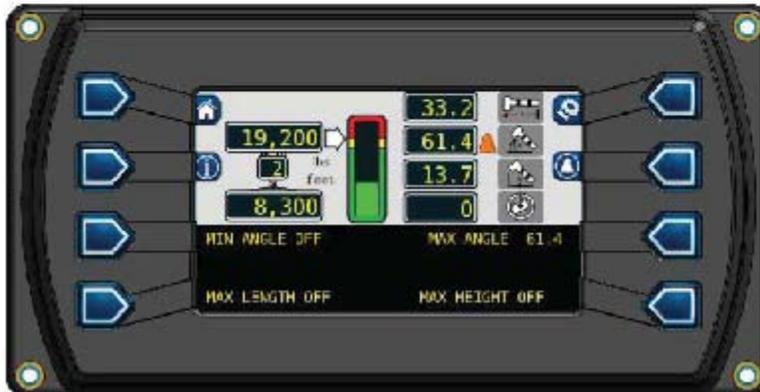
4. Pressing the MAX ANGLE button again, will cancel the alarm, and the display will read: MAX ANGLE OFF.
