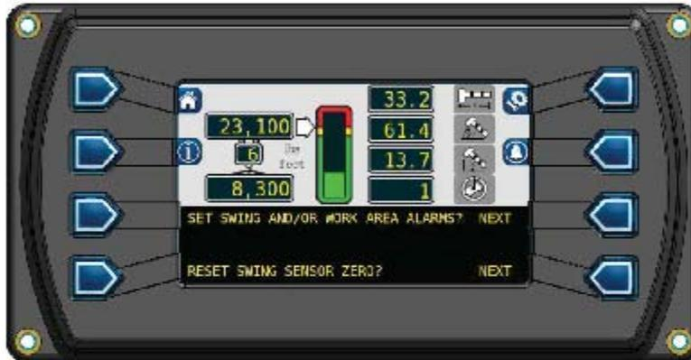
2. Ensure the boom is in its rest, (stowed position) and press the button adjacent to "CONFIRM." The swing sensor is now zeroed.
