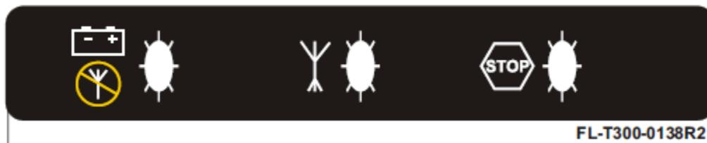
Indicator Panel lights are from left to right: Battery/Pendant, Active, E-Stop. For complete information on interpreting these lights, see section 4.2 of this manual.
