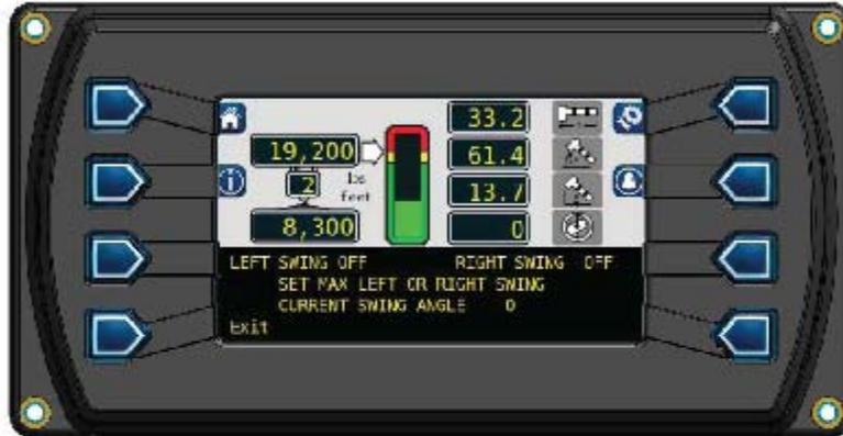
2. Next, rotate the boom to the left swing point and press the key adjacent to the "Left Swing," to set the value.
