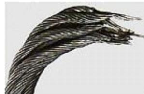
Here's a wire rope that has jumped a sheave. The rope "curled" as it went over the edge of the sheave. There are two types of breaks here: tensile "cup and cone" breaks and shear breaks that appear to have been cut on an angle.
