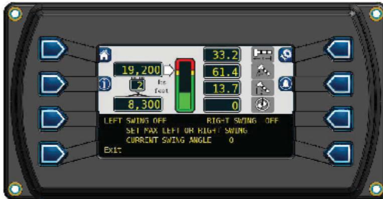
The lower buttons of the display correspond to the alarms displayed. If the alarm to be set is OFF, pressing the corresponding button will turn the alarm ON. If the alarm is ON, pressing the corresponding button once again will turn the alarm OFF.
