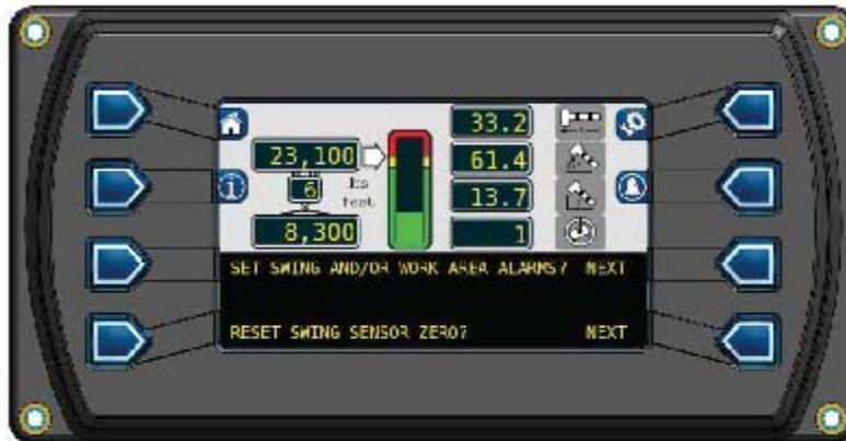
2. Press the key adjacent to the "SET LEFT AND RIGHT SWING ALARMS? SET WORKING AREA ALARM?".
