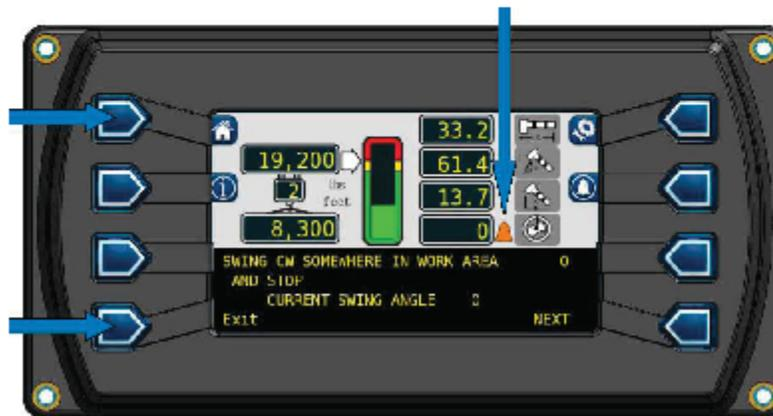
*Note: Press the operator alarm button in order to cycle through various user programmable alarms. Press the home button to return to the main screen. Exit may be chosen at any time.*
