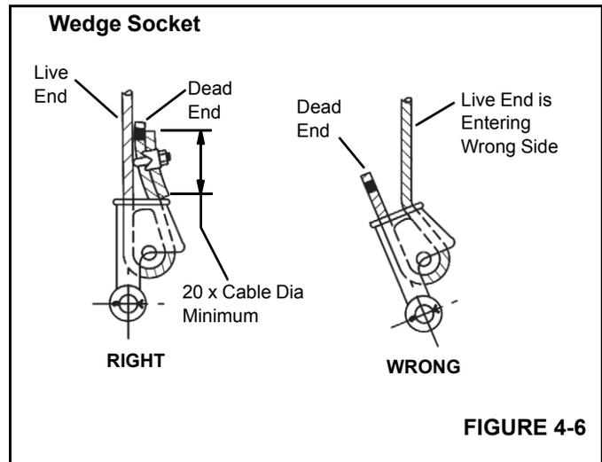
4. Insert the end of the wire rope into the socket, form a loop in the rope, and route the rope back through the socket allowing the dead-end (Figure 4-6) to protrude from the socket. Ensure the dead-end of the rope is of sufficient length to apply end treatment to the dead-end after the wedge has been seated.
