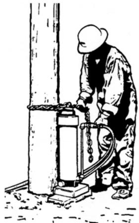
RECOMMENDED PLACEMENT OF POLE PULLER
