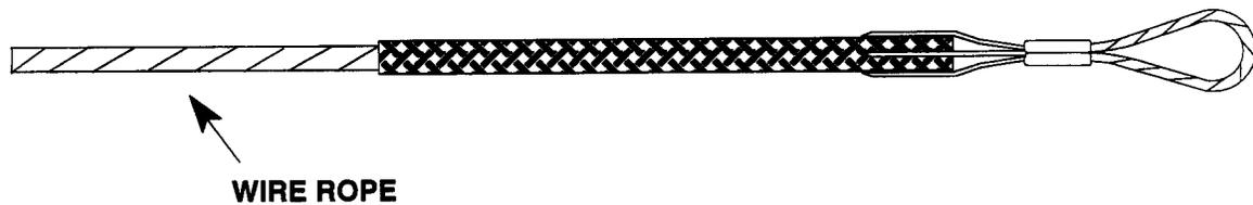
3. Release the park brake and switch the crane to Duty Cycle mode for the drum to freewheel. At the tip of the boom, pull the rope until the wire rope is to the tip.
