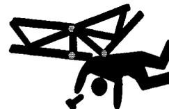
6. Always stand well clear of boom pins being removed! When the boom is on the ground on blocking, ready for disassembly, there may still be some load on individual pin connections. Under pressure from the weight of one or both of the adjoining sections, pins may fly out of their bores as they are driven out, with explosive force.
