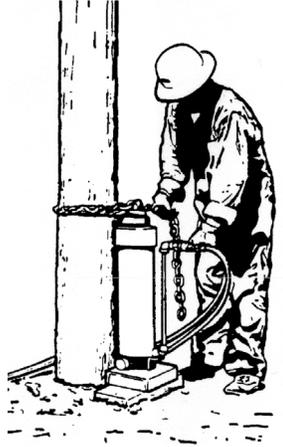
**RECOMMENDED PLACEMENT OF POLE PULLER**
