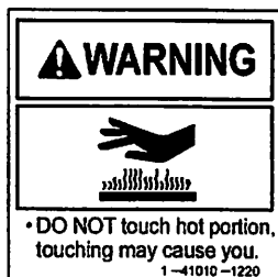
(13) Precautions for high temperature muffler (1-41010-1220)
