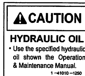
(12) Precautions for oil inside hydraulic tank (1-41010-1250)
