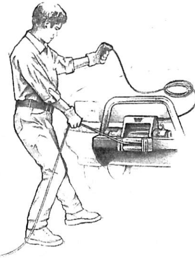
Step 18: REWIND WIRE ROPE. The person handling the wire rope should walk the rope in and not let it slide through the hand and control the winch at all times.
