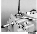
Screw Adjustable Charge Pressure Relief Valve (Motor)
