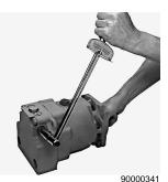
Install Flushing Shuttle Spool
