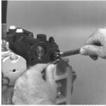
Tighten Neutral Adjusting Screw Lock Nut (Current Production HDC)
