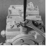
90000264 Screw Adjustable Charge Pressure Relief Valve (Pump)
