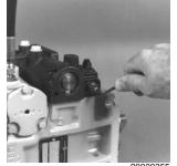
Rotate Neutral Adjusting Screw (Current Production HDC)
