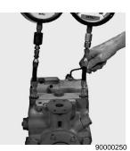
Rotate Neutral Adjusting Shaft (Early Production)
