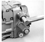
Remove Multi-Function Valve Cartridge
