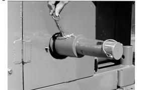
Figure 12: Polemaster Shaft Installed on the Drive
