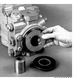
Install Spacer Plate (Intermediate Production Only)
