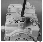
Remove Charge Relief Valve (Screw Adjustable)
