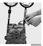
Tighten Neutral Adjusting Shaft Lock Nut (Early Production)
