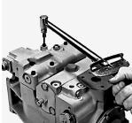
29 Torque Mounting Screws
