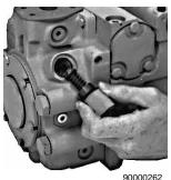
Shim Adjustable Charge Pressure Relief Valve (Pump)
