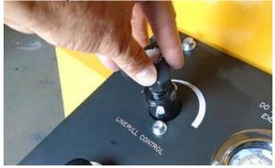
3. Brake Control - The brake is spring applied and released by hydraulic pressure also shown in Figure 3. To hold the reel stationary, turn the Reel Brake Lever to the APPLY position. Turn to the RELEASE position before driving the reel.
