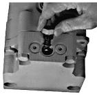
Shim Adjustable Charge Pressure Relief Valve (Motor)
