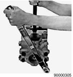
**Torque Pad Adapter** Screws
