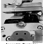
Assemble Control to Linkage
