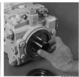
Install Charge Pump Shaft
