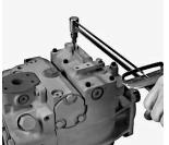
Torque Mounting Screws
