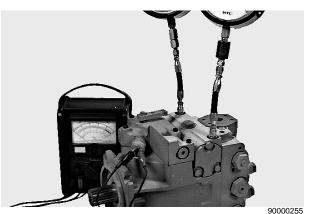
Checking Continuity of NSS (Gauges Installed in Servo Gauge Ports)
