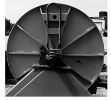
Figure 7: Lifting Loop in Vertical Position
