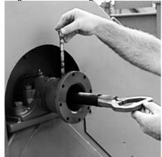
Figure 8: Removing Reel Shaft Pin
