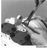
Rotate Adjusting Screw for Minimum Displacement Limiter
