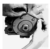
Install O-Ring on End Cap Pilot
