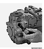
Remove Charge Relief Valve (Shim Adjustable)
