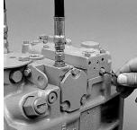
Rotate Neutral Adjusting Screw (Later Production)
