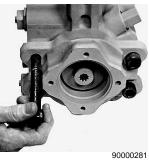
**Install Auxiliary Pad Adapter Screws**
