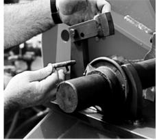
Figure 9: Removing Locking Latch
