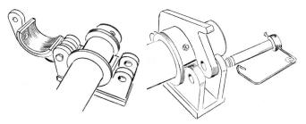
Remove the lifting device.
