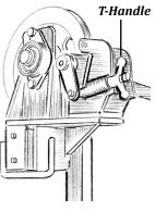
c. Engage the Tension Brake and pin it in place. Adjust the tension on the brake by turning the T-handle clockwise to increase tension as the conductor is pulled from the reel, to the desired tension level.
