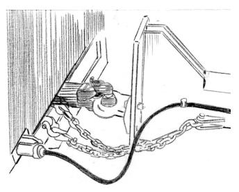
Connect the safety chains. They should be crossed and short enough to prevent the tongue from dropping to the ground if the unit should become disconnected.
