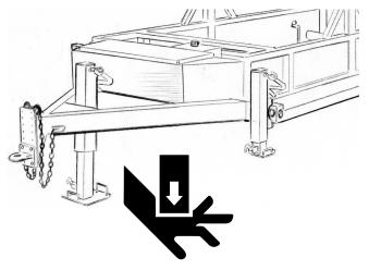
With the tow vehicle connected, make sure the hitch is securely latched.
