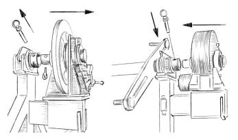
Engage the Hydraulic Retriever and pin it in position.
