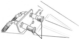
Quick Connect Hydraulic Hose Connections
