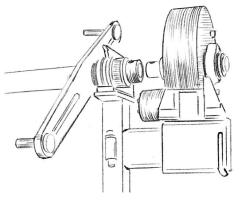
Each **Tensioning Brake** for damage, making sure the tensioning handle operates freely, and inspecting the brake pads to make sure they are serviceable. Make sure the Tensioning Brake slides in and out of the reel shaft freely, check the locking pin and retainer for damage.
