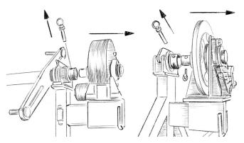
Remove the retainer and locking pin from both bearing housings and store the pin in the location provided. Open the bearing housing and remove the Reel Bar.
