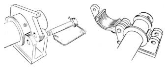
Slide the Reel Bar all of the way into the reel and make sure the two drive lugs engage the reel correctly.
