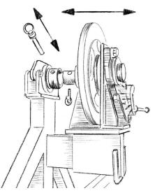
Secure any loose conductor ends on the reel.
