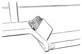
Remove the wheel chocks, place them in the holders and secure with locking device.
