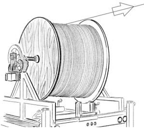
b. Unpin and disengage the Hydraulic Retriever from the reel bar.
