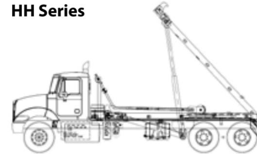
HH - A shortened and narrowed version of the OR-model that is designed to pick up deadlift containers with a knuckle cable end. The hoist rails are set at 35 inches wide.
