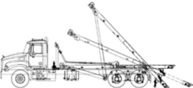
An OR-style hoist with a tail that is extendable out to an additional 48". The hoist has set rail widths of 35.5 inches.
