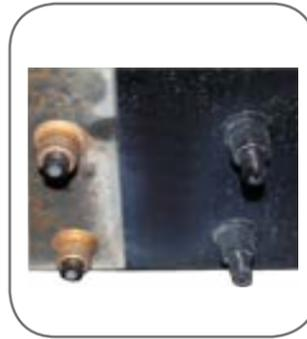
Hoist frames are huck bolted to chassis, providing unmatched strength and durability (factory mount only).
