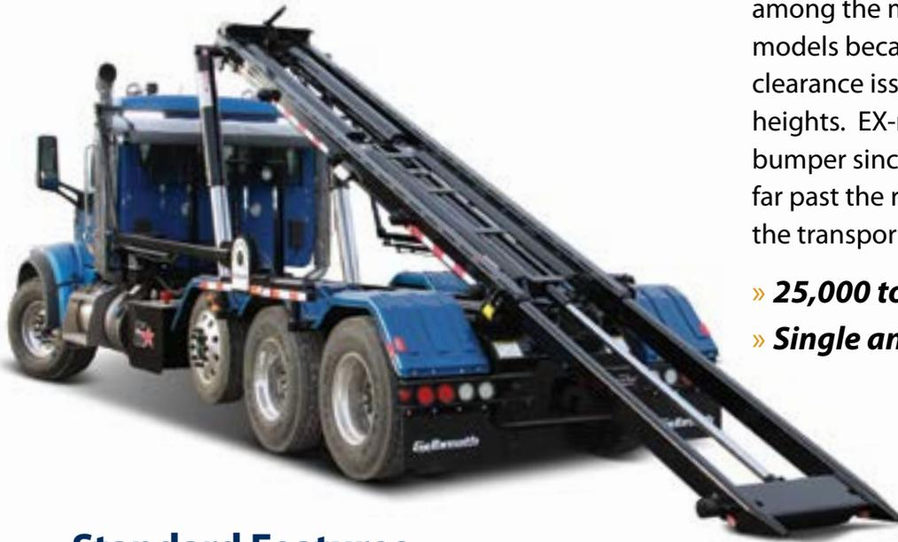
**Extendable Tail (EX)** cable hoists are among the most popular extendable tail models because they are ideal for areas with clearance issues that require low loading heights. EX-models do not require an ICC bumper since the tail does not protrude too far past the rear bumper when retracted in the transportation position.
