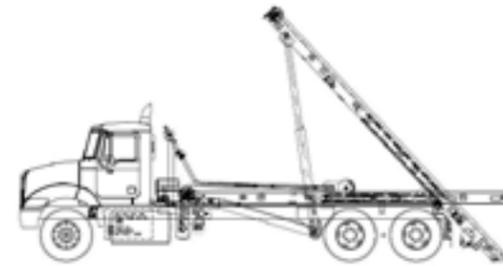
Similar to the OR-model, the IO-model has additional inside rollers (inside of main frame tubes) and inside rails fixed to the top of main frame. The hoist is set at 35.5 inches wide between rails.
