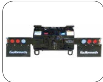
Heavy duty rear apron that comes pintle ready and a split bumper come standard on most tandem axle cable hoist models (shown with pintle hook option installed).
