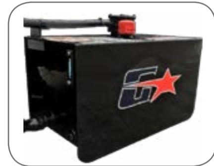
Oil reservoir equipped with 10 micron breather filter; 3 micron oil return filtration; 100 micron mesh screen suction strainer and fluid level indicator with temperature gauge.
