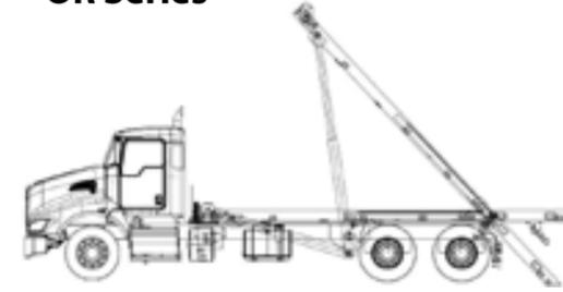
The OR-model (industry standard) is an outside/inside rail and roller hoist set at 35.5 inches wide between rails.
