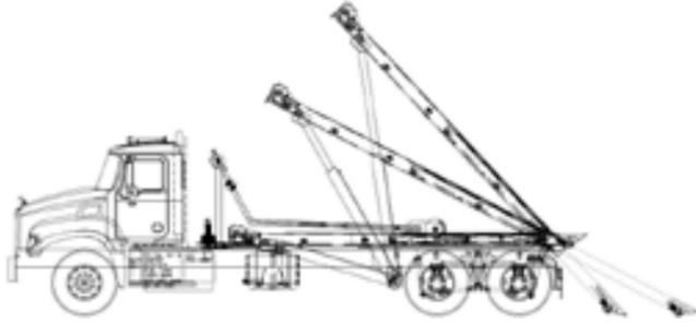
Essentially a shortened OR-model with a 80" extendable tail section that generates low loading angles and has 35.5 inch rail width.
