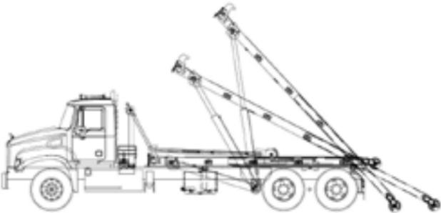
A combination of an EX & HH-model, designed for picking up dead lift containers at low loading angles with an 80" extendable tail section. This hoist has a narrower rail width set at 35 inches.
