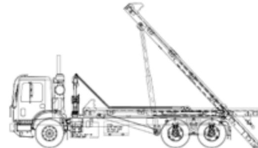
A cross breed of sorts, the SI-model is unique in the fact that it is designed to pick up a variety of different styles of containers. Specifically it will pick up either outside rail, inside/outside rail and deadlift containers. The hoist is set at 34 inches.
