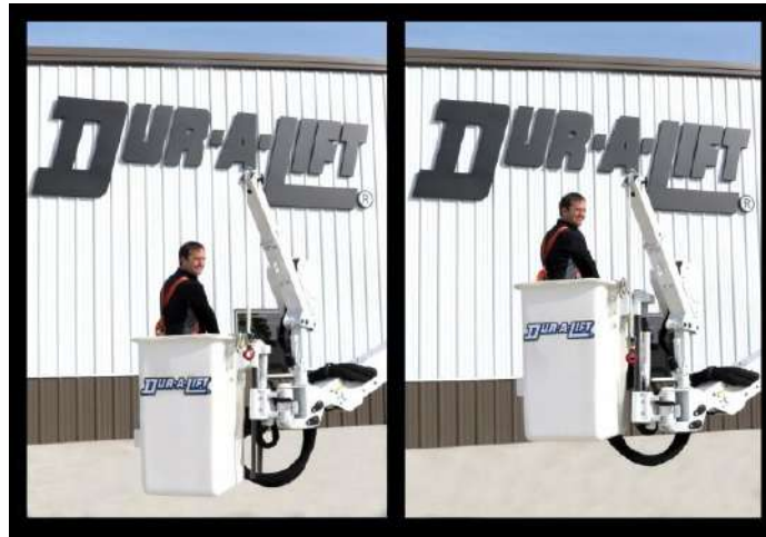
DPM2-52 Top Center Mount Winch & Jib with Elevator
