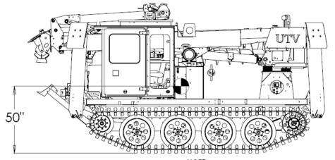
NOTE: THE C.G. HAS BEEN MEASURED USING CLOSED CAB & TIP WINCH CONFIGURATION.
